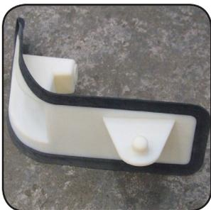
A good example was the creation of an entire telescopic headlamp washing system that extends and cleans headlamps every fifth time the windscreen is washed. The Connex-printed components proved to be robust enough for rigorous testing, allowing the design to be proved before moving into the expensive tooling stage.
