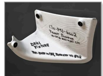
Front bumper drill fixture used to test the design.
