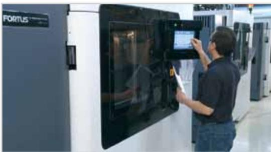
*An operator at an FDM-based Fortus Production 3-D printer.*
