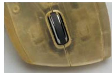
Kevin Force noted: "Our products are getting more and more complex, requiring more accurate fit testing. Being able to print fixturings, which typically need to be altered two or three times, has saved vital time and costs. Whereas fixturings were commonly made of metal and outsourced at a high cost, we can now do this in-house."
